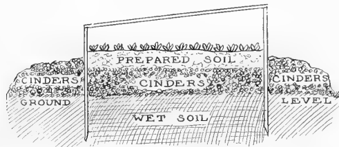
Frame prepared on wet soil, with cinder base to secure drainage
